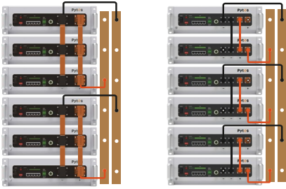
Figure 5-1 Schematic diagram of power cable connection
